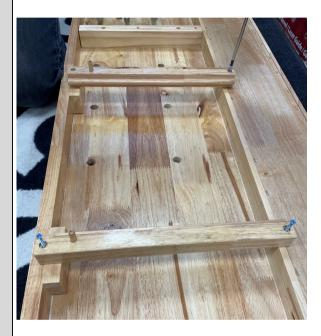
Attach the table top (4), using screws (E) & washers (C1). Insert the screws from underneath the table top (4) to secure the bench frame.
