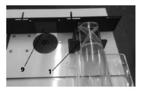
Secure the hood to the Fence base using 2 x hood screws (10), 2 x small washers
