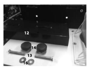
**Be aware** that the block screws fit the support block (12) to the fence base (9) through the slotted holes in the support block (12) and the circular holes in the fence base (9). Also the knob nuts (14) are used at the back of the fence base (9).
