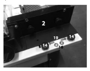
**be aware** that the screws must be inserted through the slotted hole on the table from underneath so that the knob nuts (14) can be used from the top.
