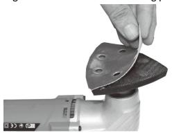
3. To remove the sanding sheet, hold it at one of the points and pull it from the sanding pad.
