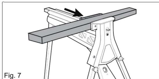
**Note:** The sliding jaw (1) can also be advanced by pressing the foot pedal (5) repeatedly.
