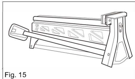
**Note:** When the Stand is in the folded position, the pull handle (11) can make it move conveniently.
