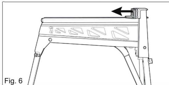
3. Carefully place your workpiece against the fixed jaw (2), while ensuring it will not fall, move the sliding jaw (1) forward by hand until it touches the workpiece.
