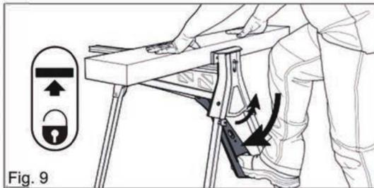
**⚠ WARNING!** Risk of injury! Ensure you are supporting the workpiece to prevent it from falling once the sliding jaw (10) is released.
