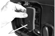
5. If the air filter is damaged contact the AUTOJACK spare parts department for a replacement.
