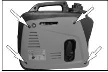
2.Remove the air filter cover screw.
