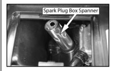
4.Remove the side panel and use the screwdriver supplied to turn the spark plug box spanner as shown.
