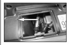
3.Fit the spark plug box spanner over the spark plug as shown.
