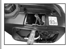
5. When the spark plug has been removed, check for discoloration and use a wire brush to remove any carbon build up.
