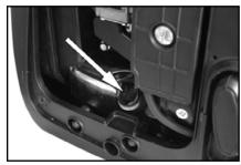
4.If the oil is below the Min. level on the dipstick, top up the oil reservoir with fresh oil.
