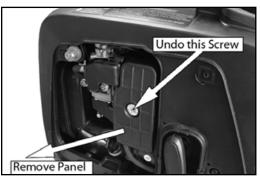
4. Remove the air filter element.
