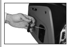
NOTE: you may have to do this more than once. WARNING: Once the generator has started, release the handle slowly to avoid injury/damage as it whips back. NOTE: When you first start the generator, the overload indicator may light up for a few seconds, this is normal. If the overload indicator is still lit after 5 seconds, stop the engine and contact your AUTOJACK dealer.
