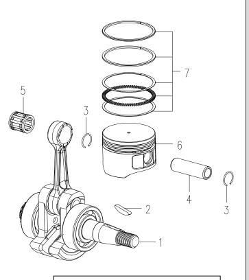
FIG. B CRANKSHAFT PISTON
