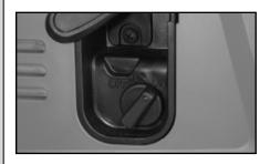
4.Set the engine switch to 'ON'.
