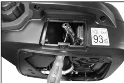
5. When the spark plug has been removed, check for discoloration and use a wire brush to remove any carbon build up.
