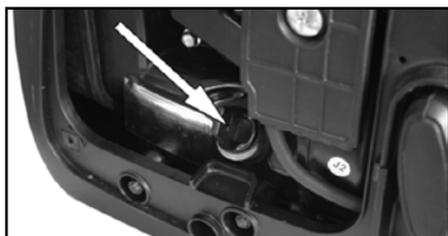
3.Tilt the generator to allow the oil to drain out of the oil reservoir into a suitable container.
