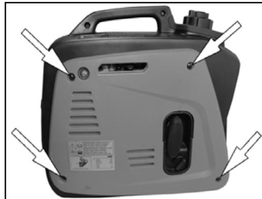
2. Remove the air filter cover screw shown on the right.
