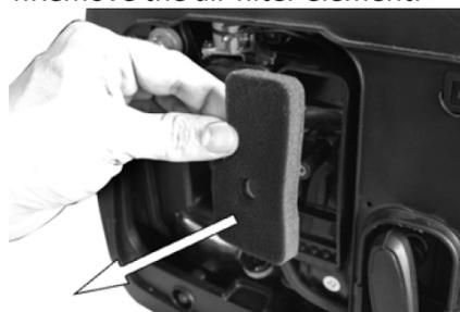
5.If the air filter is damaged contact the AUTOJACK spare parts department for a replacement.
