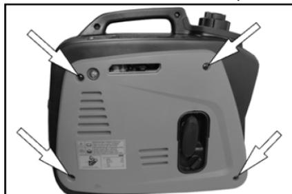
2.Remove the air filter cover screw.
