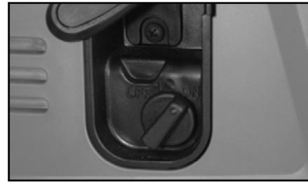
4. Set the engine switch to 'ON'.
