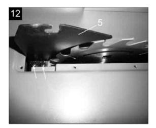
adjust the splitting wedge (5) so that the gap
