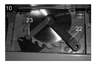
Loosen this nut and remove the flange to detach the saw blade. This needs to be pulled diagonally downwards to clear the access port.
