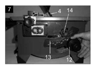
Adjust the angle of the blade by turning adjusting handle (12), until you achieve the desired angle, displayed on scale (13), and then tighten the locking handle (14) to lock the blade into position.
