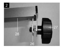
Using these claws mount the longitudinal stop
