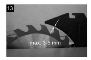
Tighten the screws holding the splitting wedge(5), then reassembly the machine.
