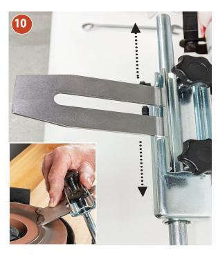
After a number of passes wipe the blade to assess the progress. A new, very bright line should appear which needs to be even across the length of the blade. If the honed edge appears one-sided simply return the guide and tool to the water stone and draw back again applying more pressure to the side with the least apparent grind. You should apply slightly more pressure to the side least ground.
