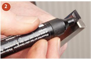
Mark the bevel with a marker to allow you to see where the grinding will occur.
