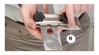
Place the tool into the jig (N) around half way along the blade and position it against the jig's stops, see fig 3. Tighten the clamping knobs. Slide the assembly onto the universal bar (M), see fig 04.
